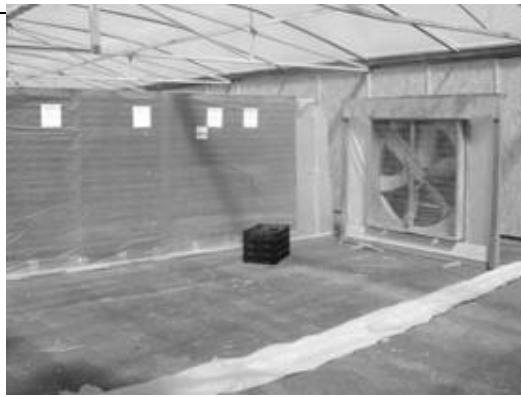
Fig. 5. Drying fan to circulate air through each individual row containing dates.
