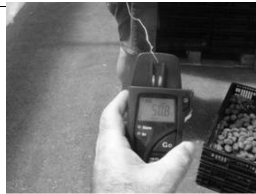
Fig. 6. Measuring 50.8°C inside dates during the disinfestation process.
